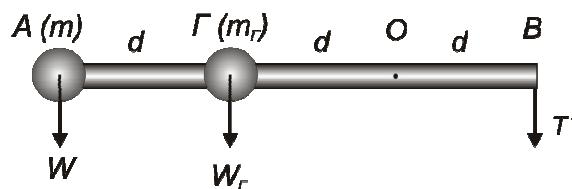
$$\Sigma \tau = 0 \Rightarrow mg2d + m_Tgd - T'd = 0 \Rightarrow mg2d = T'd - m_Tgd \Rightarrow m = \frac{T'd - m_Tgd}{g2d} \Rightarrow [m = 0,4kg]$$
